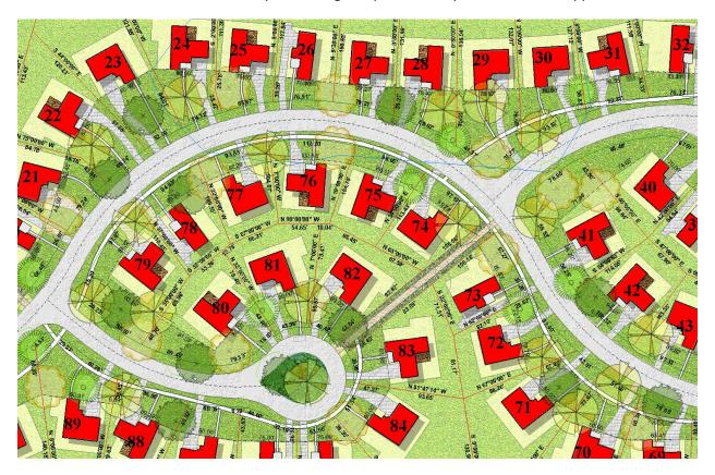
In the above example we set a 'shadow' at 135 degree angle with a 30% transparency for all 'house' surfaces. We then overlay landscaping which would typically hide dimensions and overpower the site plan, but instead set transparencies to allow dimensions to be read and not overpower the plan.
