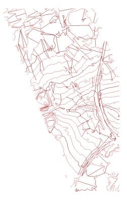
This essentially reduces the contours to emulate the land surveyors breakline data used in the design of the site delivered in less than a day's work using Landmentor as shown below.
