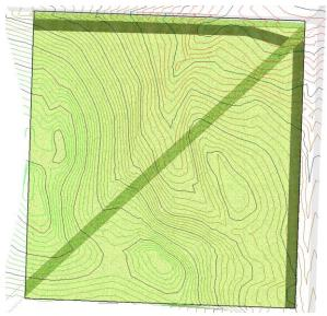
If the land is restricted by ordinance (or clients comfort level in building in slopes) to be undevelopable above 12% slope, then this slope study clearly shows that a large portion of the 'developable' land is not buildable.
