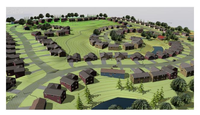
The above site was generated with less than 2,400 total points which  $1/3^{rd}$  of those points are existing ground surfaces.
