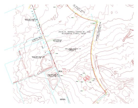
The above drawing shows contours that have been run through a 'filter' derived from LiDar. However, even filtered, there are over 43,000 points required to draw the contours. Had the data not been filtered there would have been at least a quarter million points to show the exact same topography!
