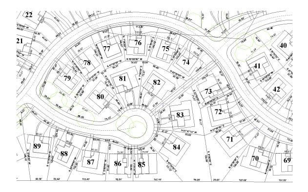
While the above is familiar, it is also difficult to decipher what is what. In CAD color variation defines line width, but in LandMentor line width is accurately displayed and color = color, significantly reducing mental gymnastics. Varying line width helps separate some data:
