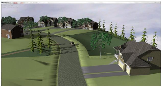
The ground abutting the street shows the proposed grading detail derived by the proposed DTM. In LandMentor while in the Video Gaming window, pressing [W] allows the wirelines that created the 3D to appear...
